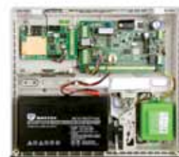
CS47 Link BD Internal card to be installed into the Runner™ Control Panel housing
